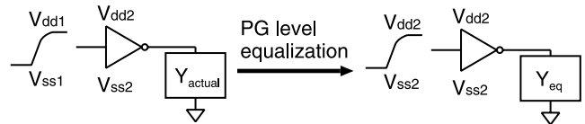
Fig. 15 PG level equalization for generic load.
