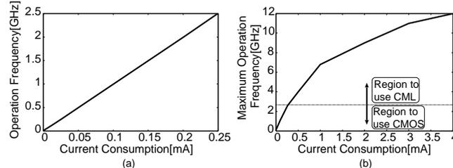
Fig. 2. Operating Frequency vs. Current of a divider: (a) CMOS Static Logic, (b) CML.
