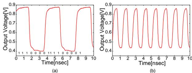
Fig. 5. Measured output waveform ( $\text{IN}_0\text{-IN}_7$ :10101001): (a) 2Gbps, (b) 6.4Gbps.
