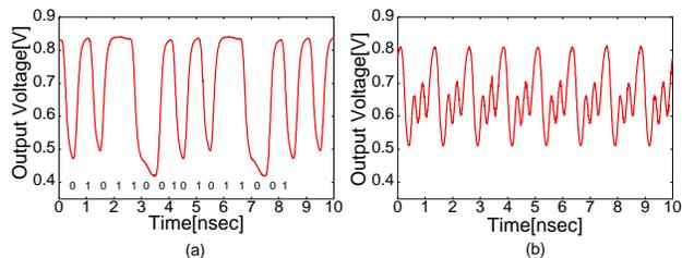
Fig. 6. Measured output waveform ( $\text{IN}_0\text{-IN}_7$ :01001011): (a) 2Gbps, (b) 6.4Gbps.
