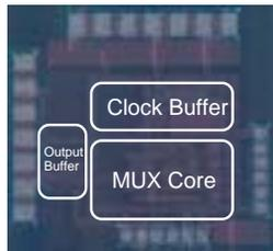
Fig. 4. Chip photograph of hybrid 8:1 MUX.
