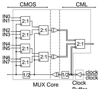
Fig. 3. Configuration of hybrid 8:1 MUX.
