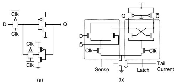
Fig. 1. Schematic of D-latch : (a) CMOS static logic, (b) CML.
