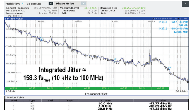
Fig. 22. Measured THz source phase noise at 318.21 GHz.
