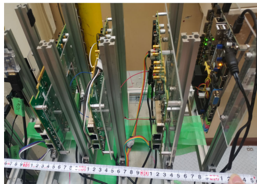
Fig. 11. Experimental setup for neutron irradiation at CYRIC, Tohoku University.
