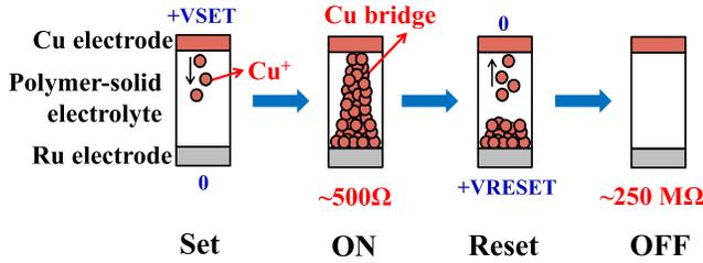
Fig. 3. Set/reset operations of an AS.
