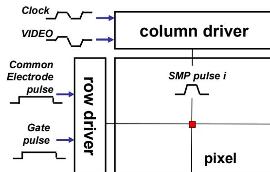
Fig. 1: An active matrix LCD
