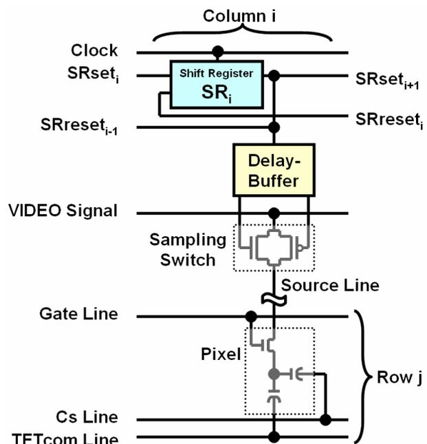
Fig. 2: A circuit for a column of the column driver in active matrix LCD
