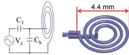
Fig. 10. Antenna with a coil and two capacitors and its simulation model.
