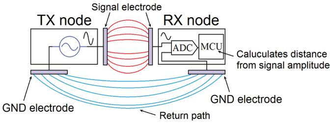
Fig. 2. Distance sensing based on capacitive coupling.
