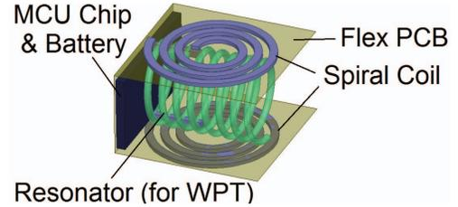
Fig. 4. Accommodating helical coil resonator for wireless power transfer and proposed dual-use antenna in a sensor node.
