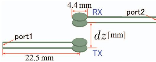
Fig. 9. Simulation model with disc electrodes in distance sensing mode.
