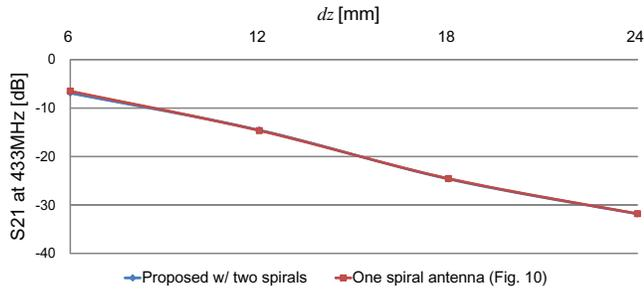
Fig. 13. S21 comparison between proposed antenna and Fig. 10.
