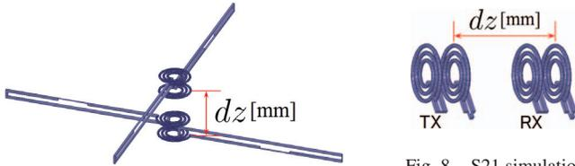
Fig. 7. S21 simulation model with lead wire.
