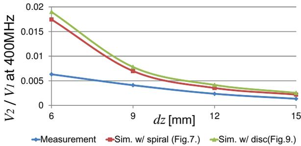
Fig. 15. Measured and simulated  $V_2/V_1$  in distance sensing mode.
