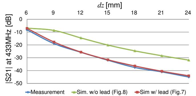
Fig. 12. Measured and simulated S21 results in communication mode.
