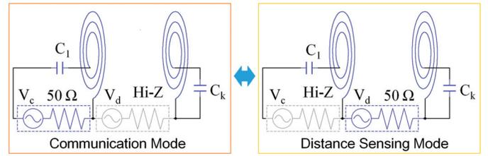
Fig. 3. Proposed dual-use antenna providing two function modes.
