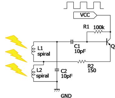
Fig. 6. Proposed transmitter.
