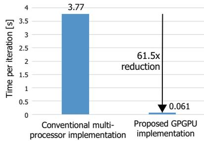
Fig. 2. Acceleration thanks to GPU implementation of 3D node localization.
