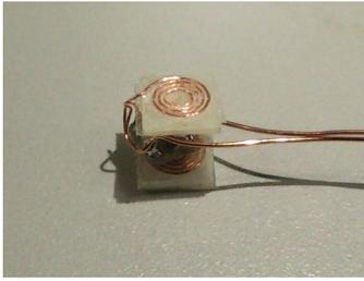
Fig. 7. Prototype of proposed transmitter.
