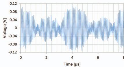
Fig. 11. Waveform at receiver in case of 1Mbps communication.
