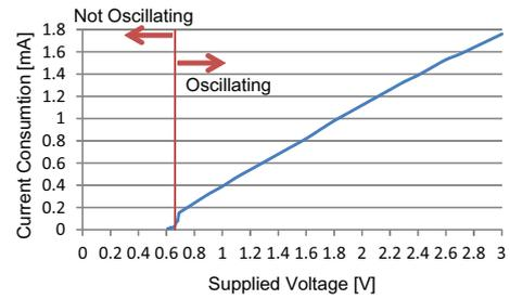
Fig. 9. Current consumption versus supply voltage.
