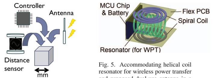
Fig. 4. Difficulty in integrating multiple devices into a small volume.
