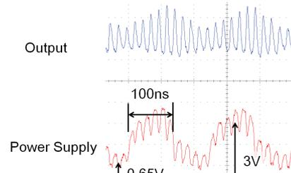
Fig. 10. Transmitter output for 3 V, 20 Mbps communication.
