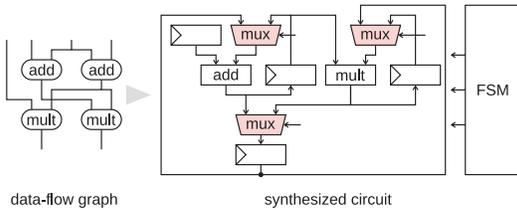
Fig. 5. MUXes for resource sharing generated by high-level synthesis.
