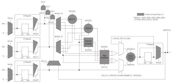
Fig. 4. Block diagram of the arithmetic block (AB) [4].
