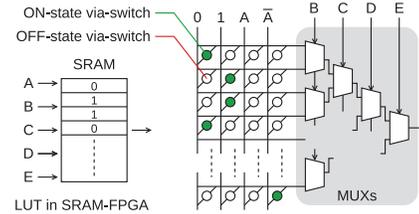
Fig. 3. LUT in VS-FPGA ( $0/1/A/\bar{A}$ -type LUT) [7].
