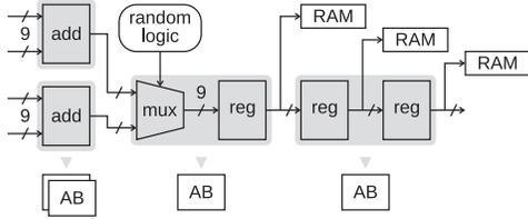
Fig. 6. A typical example of a control circuit.
