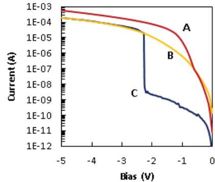
Fig. 8 I-V characteristics of Ge<sub>x</sub>Se<sub>1-x</sub> films
