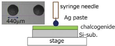
Fig. 4 Printed upper electrodes
