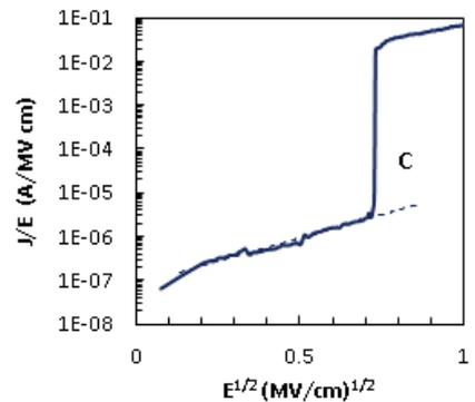
Fig. 9 Analysis of off-state I-V characteristics (Poole-Frenkel conduction)
