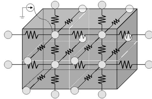
Figure 5. An example of heat diffusion model.
