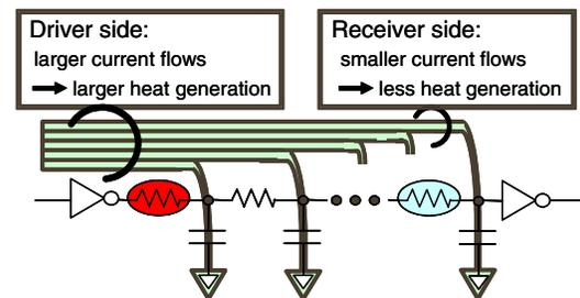
Figure 6. Nonuniform heating in a wire.
