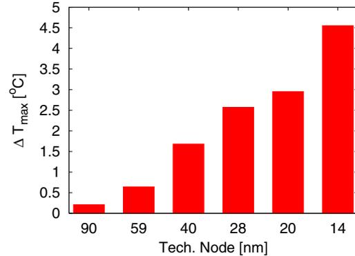
**Figure 11. Prediction result of temperature rise from the ambient,  $\Delta T_{max}$  (global wire).**
