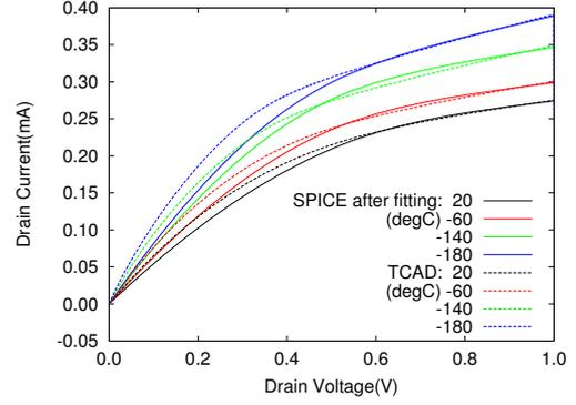
Fig. 2. Fitting results of NMOS  $V_d - I_d$  characteristics.
