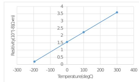
Fig. 1. Temperature dependency of the volume resistivity of copper
