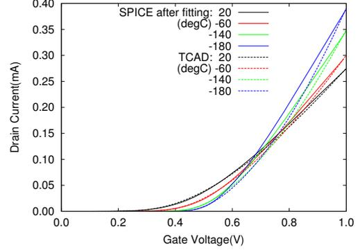
Fig. 3. Fitting results of NMOS  $V_g - I_d$  characteristics.
