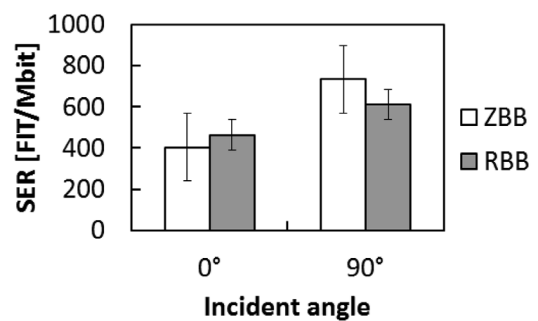
Fig. 11. Measured MCU rates of bulk SRAM at 0.4 V.
