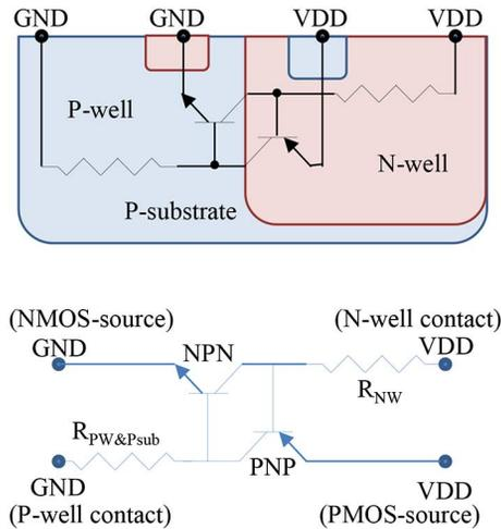
Fig. 1. Schematic of parasitic bipolar transistors contributing to SEL in a typical CMOS structure.
