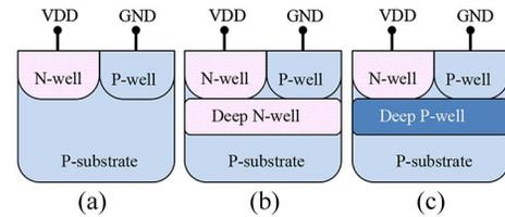
Fig. 2. Well configurations; (a) twin-well (2 W), (b) ordinary triple-well with deep N-well (DNW) and (c) with deep P-well (DPW). (a) w/o DW(twin-well) (b) w/ DNW(triple-well) (c) w/DPW.
