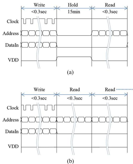
Fig. 3. Two types of test; (a) static and (b) dynamic tests.
