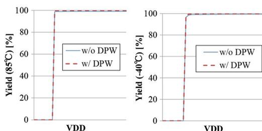
Fig. 14. Chip level yields measured by wafer level test in 85 and -40 degree Celsius.
