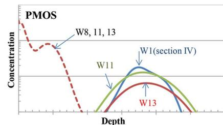
Fig. 9. N-well and DPW profiles of wafer of W1, W8, W11, W13. Right mountain-like curves correspond to DPW.
