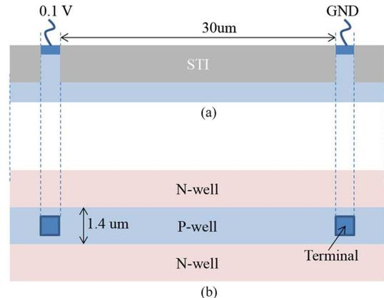
Fig. 11. (a) cross section and (b) top view of P-well resistor monitor.
