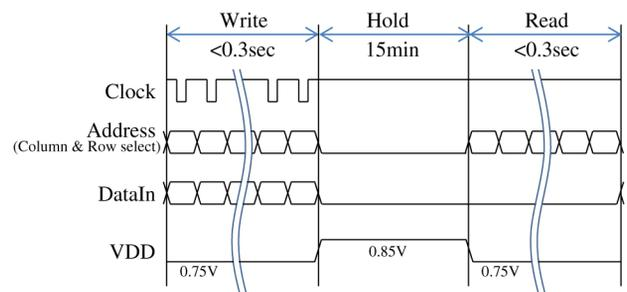
Fig. 11. Test timing chart.
