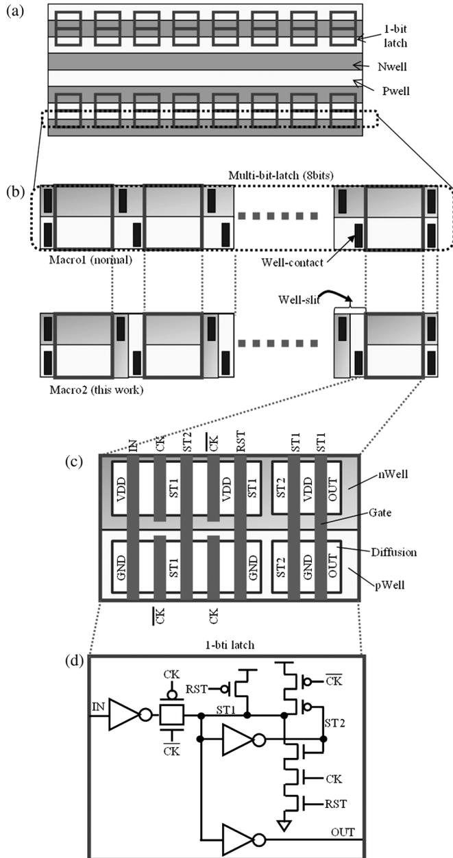
Fig. 6. (a) MBL macro placement on the test chip, (b) layout of 8-bit MBL of two macros on test chip, (c) latch layout and (d) schematic of 1-bit latch.
