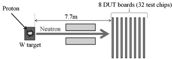
Fig. 5. Neutron test configuration at RCNP.
