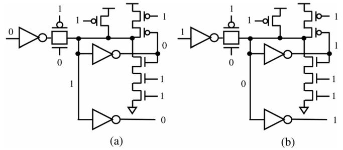
Fig. 7. Node values when retention data is (a) 0 and (b) 1. The input data of the latches are the same with written data during hold operation.
