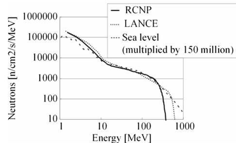
Fig. 4. Neutron spectrum at sea level (multiplied by 150 million) and spectrums on of spallation neutron beams at RCNP and LANCE [9].
