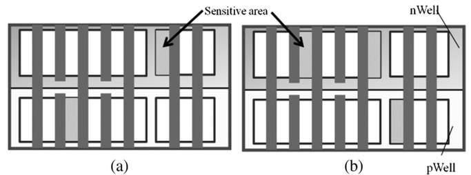
Fig. 8. Sensitive area when retention data is (a) 0 and (b) 1.
