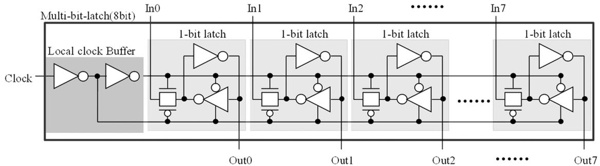
Fig. 2. Multi-bit-latch with clock buffer (8-bit).
