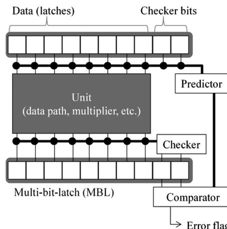
Fig. 1. Circuits necessary for HIR.
