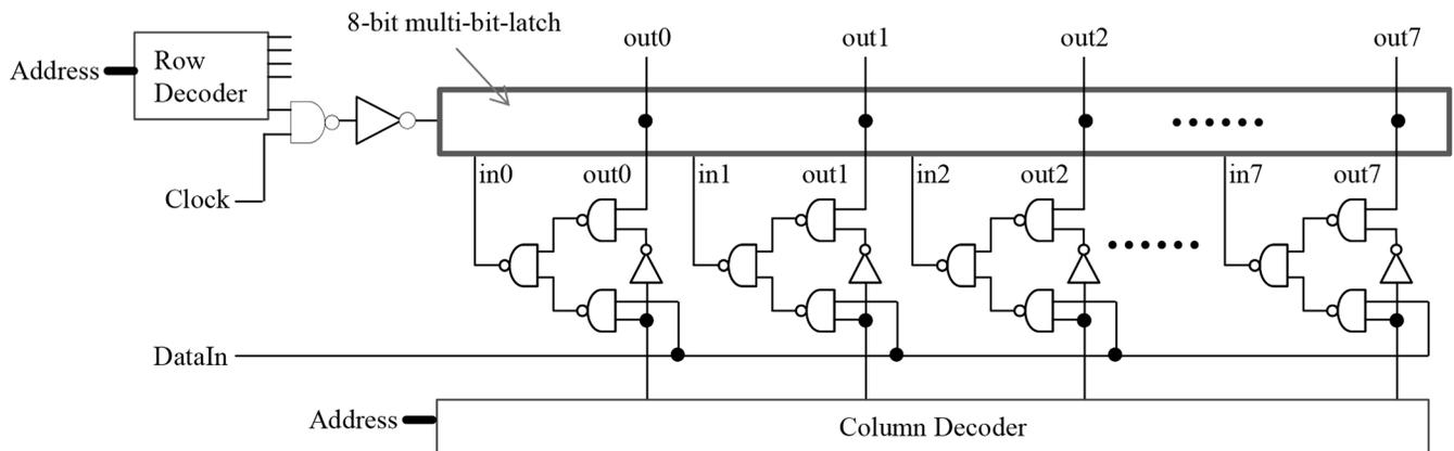
Fig. 10. Control logic for 8-bit MBL in the test chip.
