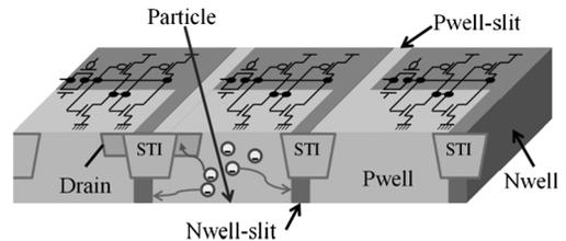
Fig. 3. Proposed MBU mitigation technique using well-slit for MBL.
