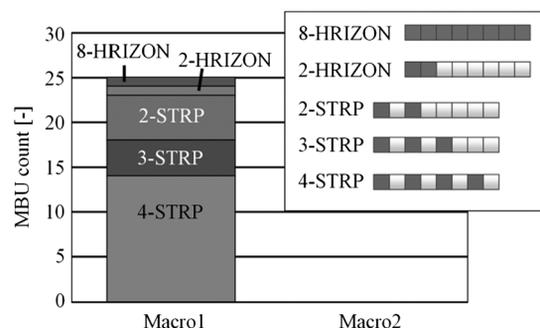
Fig. 13. MBU counts in neutron irradiation test on macro1 (normal) and macro2 (with well-slit) of 28 nm latches.
