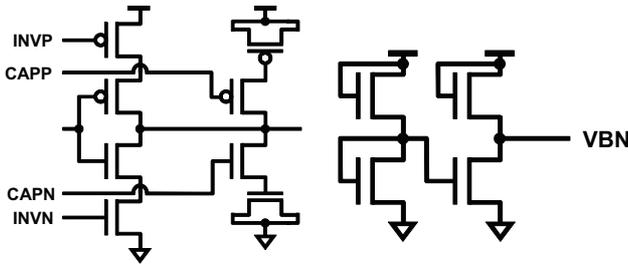
Fig. 2. Single inverting stage for sensitivity-configurable RO.
