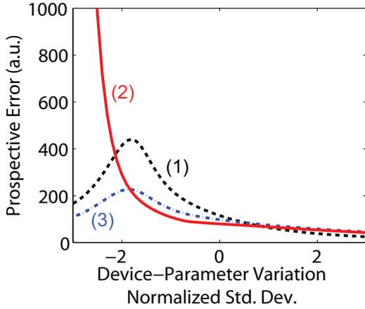
Fig. 1. The best combination varies in device-parameter space. Each of three lines (1) – (3) corresponds to a combination of sensitivity configurations. X-axis expresses a representative device-parameter variation normalized by its standard deviation.
