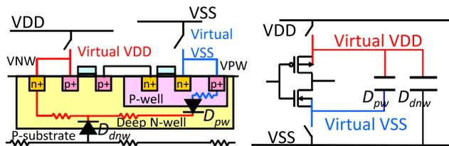
Fig. 1 Cross-section and circuit representation of triple-well structure with body-gated option.
