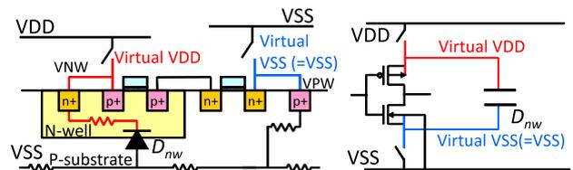
Fig. 2 Cross-section and circuit representation of twin-well structure with body-gated option.
