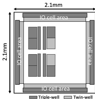
Fig. 12 Well layout of test chip.
