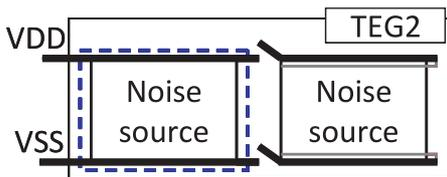
Fig. 8 TEG2: triple-well to twin-well, body-gated. Dotted line represents deep N-well, bold lines are VDD and VSS lines, and gray lines show body connection.
