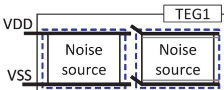
Fig. 7 TEG1: triple-well to triple-well, body-gated. Dotted line represents deep N-well, bold lines are VDD and VSS lines, and gray lines show body connection.
