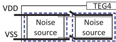
Fig. 10 TEG4: triple-well to triple-well, body-tied. Dotted line represents deep N-well, bold lines are VDD and VSS lines, and gray lines show body connection.
