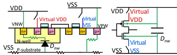
Fig. 3 Cross-section and circuit representation of twin-well structure with body-tied option.
