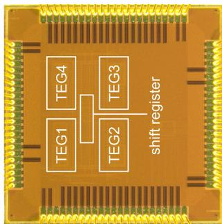
Fig. 5 Chip micrograph (2.1 mm × 2.1 mm).
