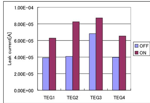
**Fig. 15** Measured leakage currents when gating switch is ON or OFF.
