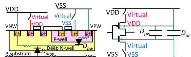
Fig. 4 Cross-section and circuit representation of triple-well structure with body-tied option.
