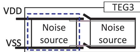
Fig. 9 TEG3: triple-well to twin-well, body-tied. Dotted line represents deep N-well, bold lines are VDD and VSS lines, and gray lines show body connection.
