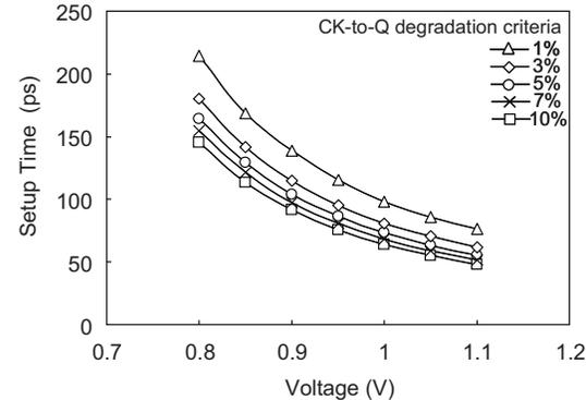
Fig. 4. Setup time dependence on supply voltage.
