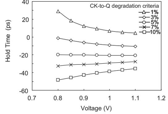
Fig. 5. Hold time dependence on supply voltage.
