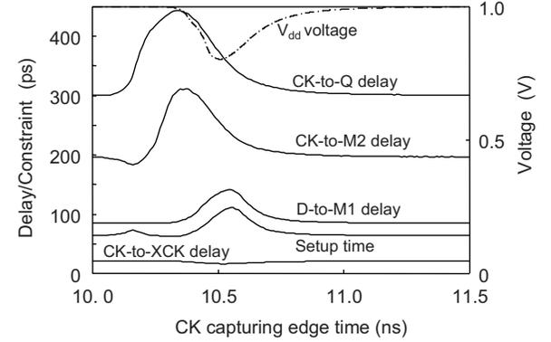
Fig. 6. Setup time dependence on dynamic voltage drop.
