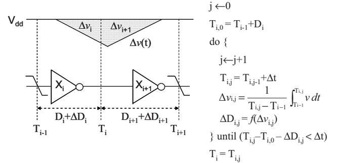
Fig. 7. An iterative procedure to obtain stage delay increase from voltage-delay characteristics.
