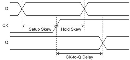
Fig. 2. Timing definitions of setup/hold skews.
