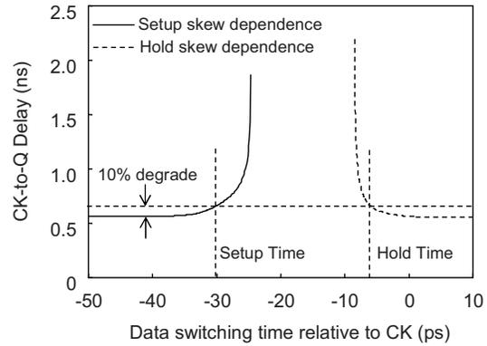
Fig. 3. Relation between CK-to-Q delay and setup/hold skews.
