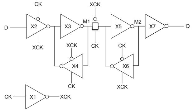
Fig. 1. Circuit diagram of Flip-Flop.
