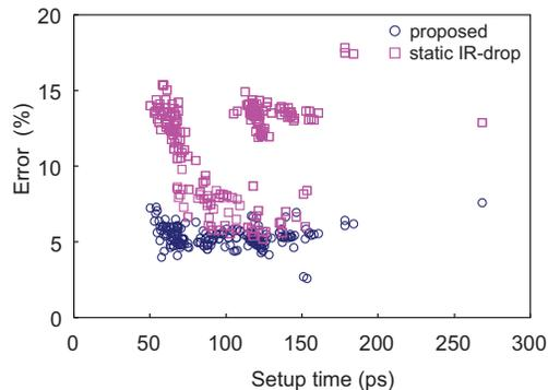
Fig. 9. Accuracy evaluation results of setup time estimation.
