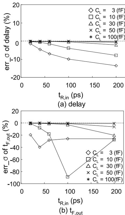
**Fig. 6**  $err_{\sigma}$  (%) of the estimated distribution by the linear correlation of NMOS threshold voltage: (a) Delay time distribution. (b) Output transition-time distribution.
