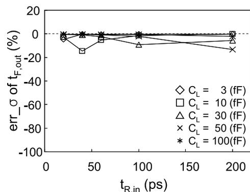
Fig. 11  $err_{\sigma}$  (%) of the estimated output transition time distribution by our proposed method.
