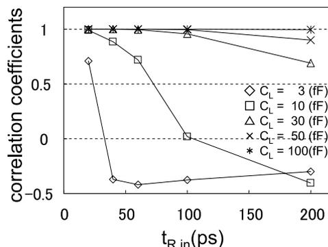
Fig. 2 Correlation coefficients between delay and output transition time under the combinations of input transition time ( $t_{R,in}$ ) and output load ( $C_L$ ) in Table 1.
