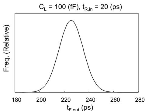
**Fig. 5** Computed result of the output transition-time distribution by the approximated linear correlation in the high correlation case of Fig. 3(a).
