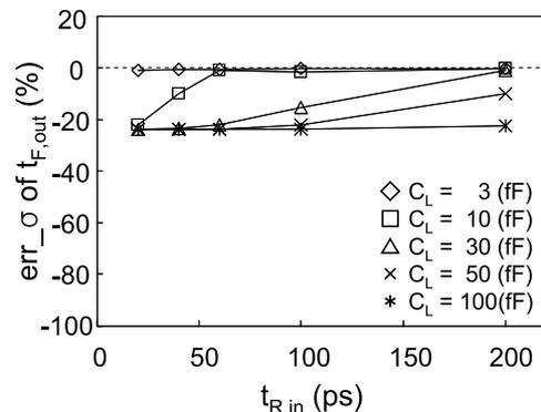
Fig. 9  $err_{\sigma}$  (%) of the estimated output transition-time distribution by the quadratic relation of  $V_{margin}$ .
