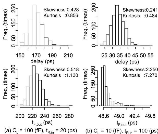
Fig. 3 Distributions of delay and output transition-time dependent on the correlation between delay and output transition-time: (a) High correlation combination case. (b) Low correlation combination case.
