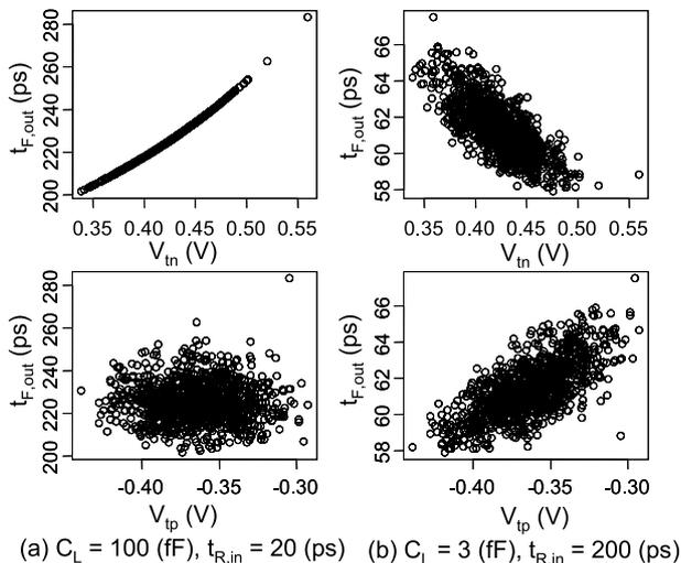
**Fig. 4** Scatter plot of output transition-time and NMOS/PMOS threshold voltages dependent on the correlation between delay and output transition-time: (a) High correlation combination case. (b) Low correlation combination case.
