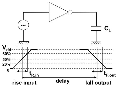
Fig. 1 Experimental circuit setup and timing definitions.
