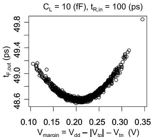
Fig. 7 Scatter plot of output transition-time and voltage margin ( $V_{margin}$ ).
