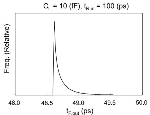
Fig. 8 Computed result of the output transition-time distribution by the approximated quadratic relation in the low correlation case of Fig. 3(b).
