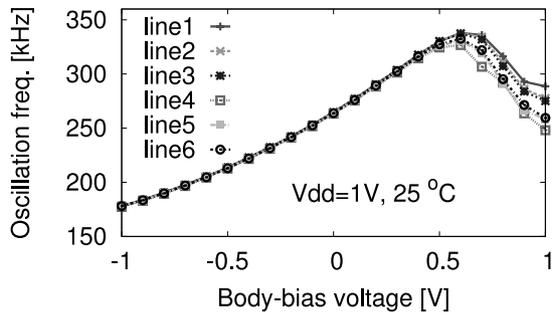
Fig. 4 Measured frequency of ring oscillator at  $V_{dd} = 1\text{ V}$  and  $25^\circ\text{C}$ .
