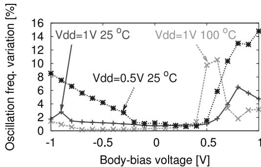
Fig. 5 Frequency variation among lines at  $\{V_{dd} = 1\text{ V}, 25^\circ\text{C}\}$ ,  $\{V_{dd} = 1\text{ V}, 100^\circ\text{C}\}$  and  $\{V_{dd} = 0.5\text{ V}, 25^\circ\text{C}\}$ .
