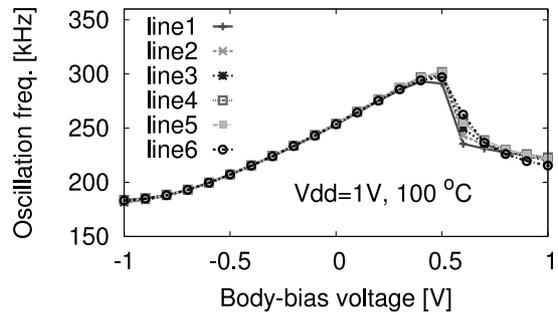
Fig. 6 Measured frequency of ring oscillator at  $V_{dd} = 1\text{ V}$  and  $100^\circ\text{C}$ .
