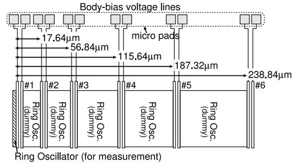
**Fig. 2** Structure of test circuit.
