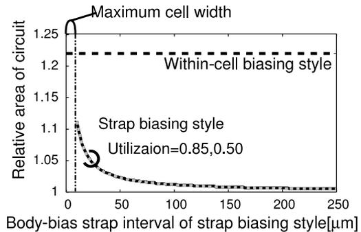
**Fig. 9** Area efficiency of strap biasing style with varied strap intervals (curved lines). Horizontal dashed line corresponds to within-cell biasing style.
