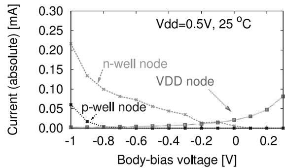
Fig. 8 Measured current at  $V_{dd} = 0.5\text{ V}$  and  $25^\circ\text{C}$ .
