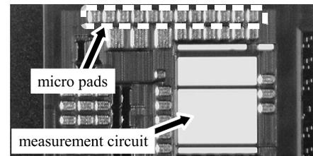
**Fig. 3** Micrograph of fabricated test chip.
