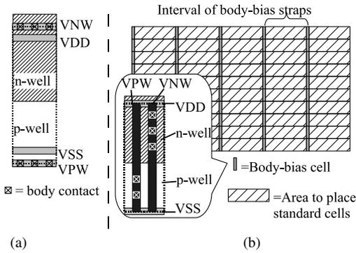
**Fig. 1** Cell layout for body-biasing. (a) Within-cell biasing style, (b) Strap biasing style.
