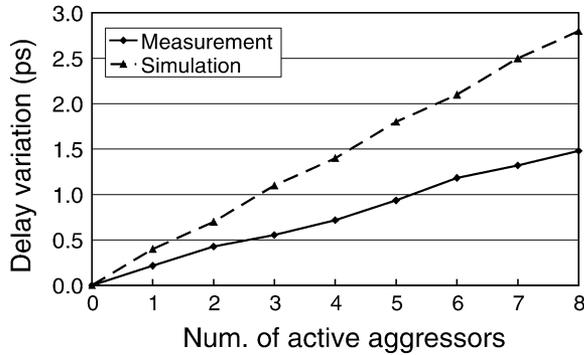
Fig. 17. Measurement results for delay change on TEG\_STD at aggressor timing = 180 ps.
