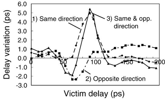
Fig. 31. Timing of opposite direction transition is shifted from Fig. 30.
