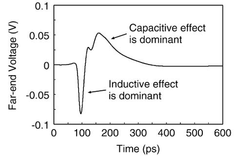
Fig. 3. A coupling noise waveform.
