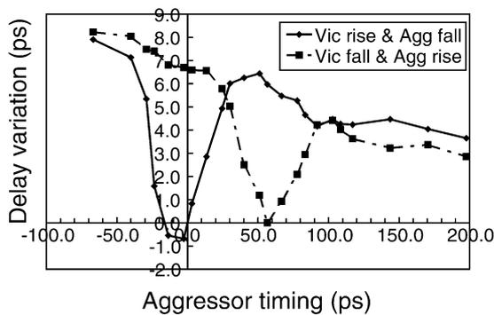
Fig. 18. Measurement results for delay change on TEG\_STD. Transition directions of aggressors are opposite to those of the victim.
