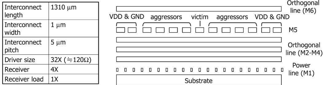
Fig. 12. Interconnect cross section.
