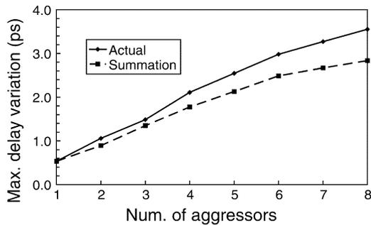
Fig. 7. Interconnect delay variation due to inductive coupling noise was simulated with MOS drivers. Delay variation of overlapped noise, and summation of delay variation due to each individual noise are compared.
