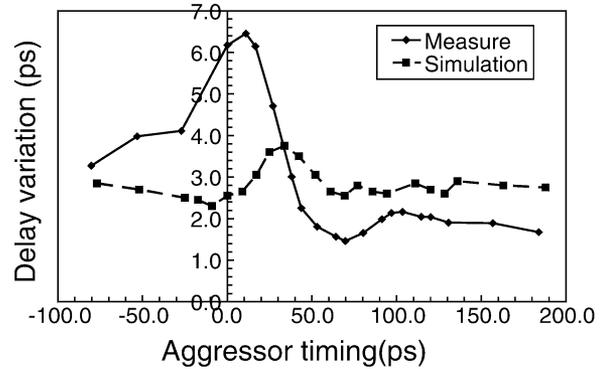
Fig. 25. Comparison between measurement and simulation results of TEG.M2POWERLINE.
