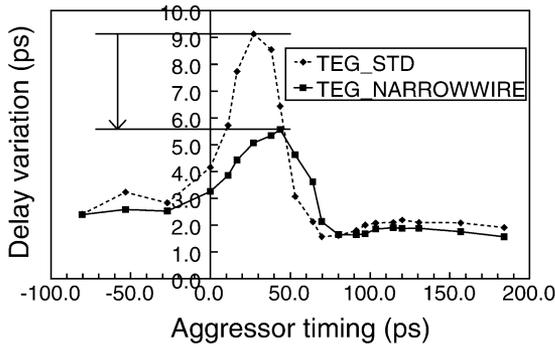
Fig. 21. Measurement of TEG.NARROWWIRE. Narrow signal wires damp inductive noise.
