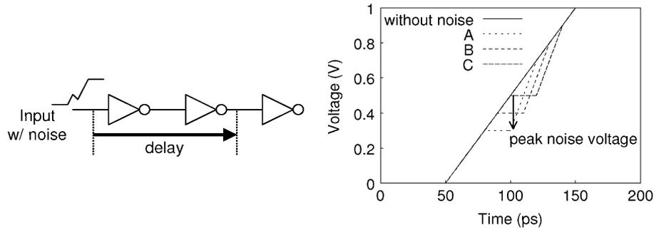
Fig. 5. Simulation setup of Fig. 6. Figure on left is circuit for simulation. All inverters are same size. Graph on right is inverter input voltage waveform of the three graphs in Fig. 6.
