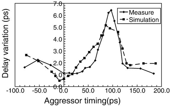
Fig. 27. Comparison between measurement and simulation results of TEG\_SMALLDRIVE.
