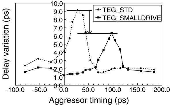
Fig. 22. Measurement of TEG.SMALLDRIVE. Small driver injects less noise.
