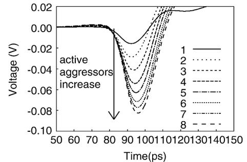
Fig. 4. Overlapped noise waveform simulated with resistive drivers. Number of key is number of active aggressors. Each aggressor makes rise transition at same timing.
