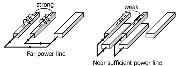
Fig. 1. Dependence of inductive coupling on power lines.
