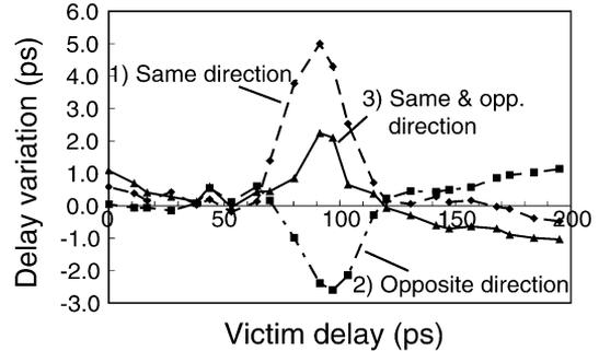
Fig. 30. Measurement results when aggressors make same and/or opposite direction transition.
