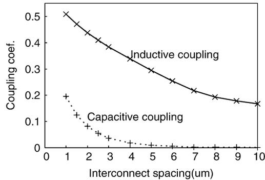
Fig. 13. Interconnect spacing and coupling coefficient. Inductive and capacitive coupling coefficients are normalized with coefficients at 1  $\mu\text{m}$  spacing respectively.
