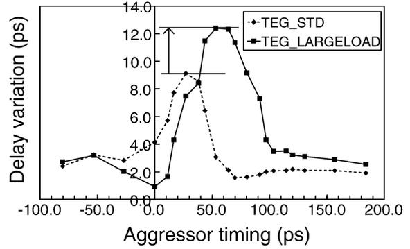
Fig. 23. Measurement of TEG.LARGELOAD. Large receiver load enlarges noise susceptible timing.
