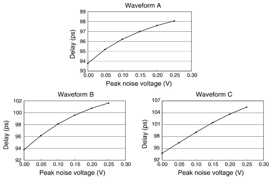
Fig. 6. Noise peak voltage of inverter input and propagation delay in simulation. X axis is the peak noise voltage.
