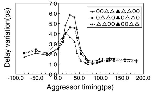
Fig. 19. Measurement result for delay change when four near/far aggressors are active. "0" is an inactive aggressor, and "△" is an active aggressor. "▲" at the center corresponds to the victim.
