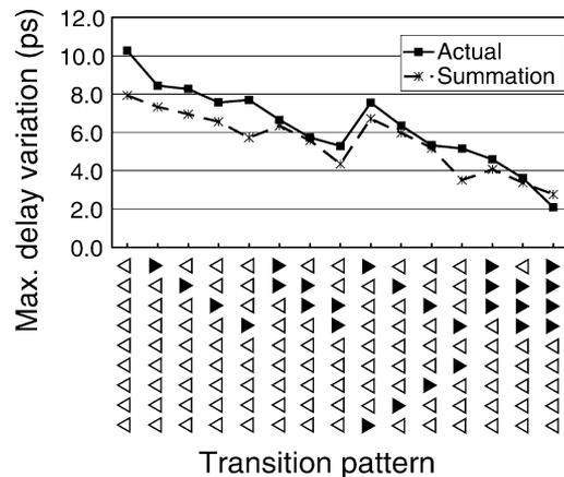
Fig. 33. Measured maximum delay variation due to inductive coupling including opposite direction transitions. Delay variations of overlapped noise and summation of each individual noise are compared.
