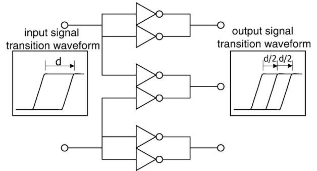
Fig. 11. Phase interpolator.
