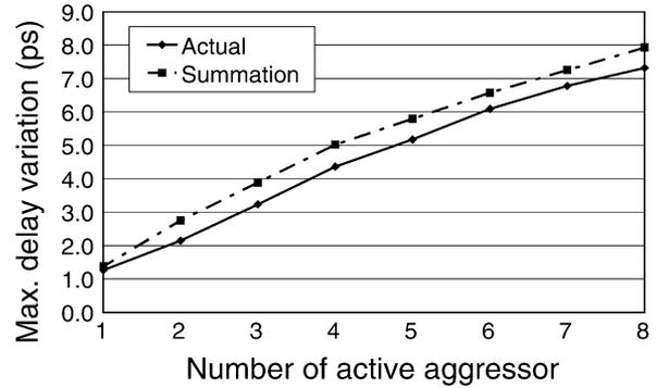
Fig. 32. Measured maximum delay variation due to inductive coupling. Delay variations of overlapped noise and summation of individual noises are compared.
