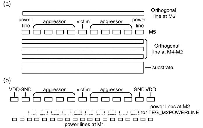
Fig. 15. Interconnect structure for  $RLC$  extraction.
