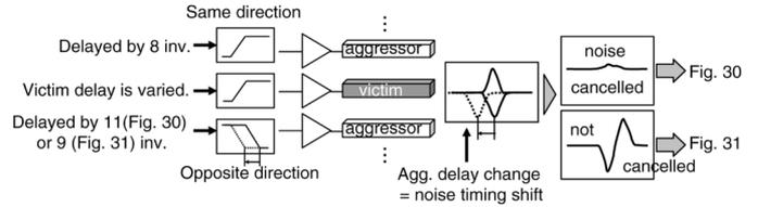
Fig. 29. Measurement setup of Figs. 30 and 31. Same and opposite direction transition are input to aggressors to observe noise cancellation effect.
