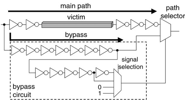
Fig. 10. Bypass circuit.
