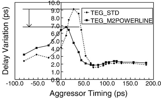
Fig. 20. Measurement of TEG.M2POWERLINE. Parallel wires in M2 weakened inductive coupling.
