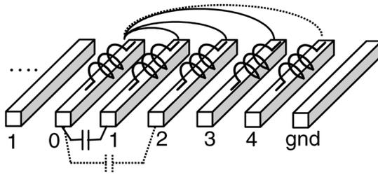
Fig. 2. Long-range effect of inductive coupling.
