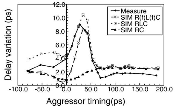
Fig. 16. Delay change due to coupling noise on TEG-STD.
